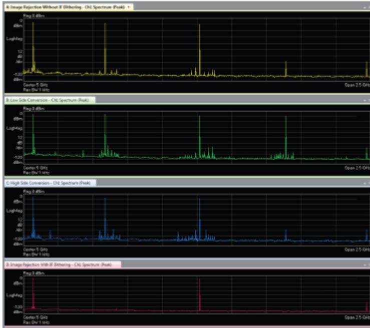
**Figure 10. The combination of IF dithering and image rejection produces a frequency spectrum with only real components at 4.02 GHz and 5.22 GHz.**
