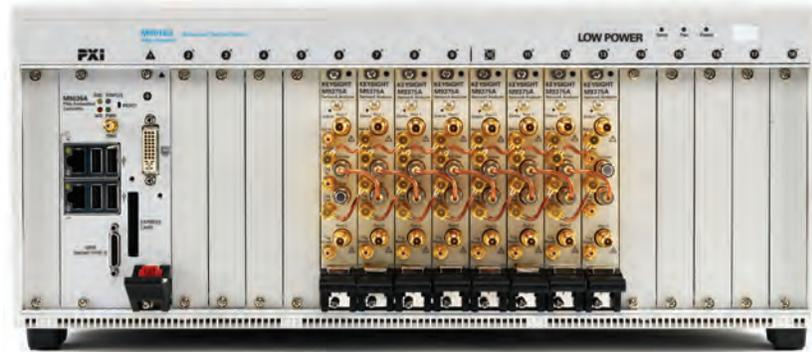
FIGURE 2. This versatile multi-port configuration uses eight two-port PXI VNAs in a single chassis.
