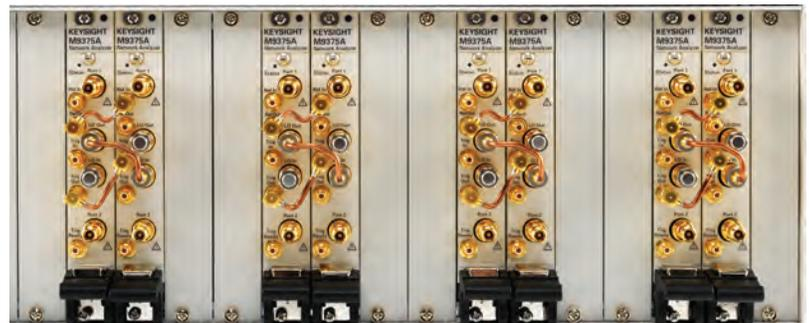
FIGURE 3. This example multi-site configuration includes a quartet of independent four-port PXI VNAs in a single chassis.
