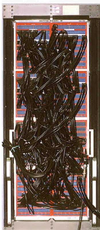
*Figure 2. Traditional Fault Insertion System Using a Patch Panel to Inject Faults Manually*
