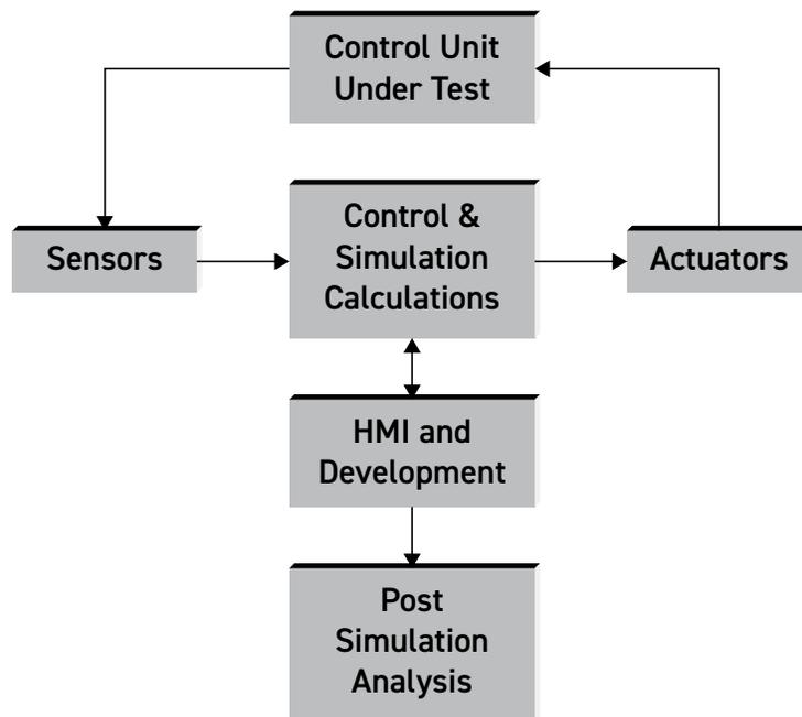
Figure 1. HILS Model Showing the Simulation of an Operating Environment
