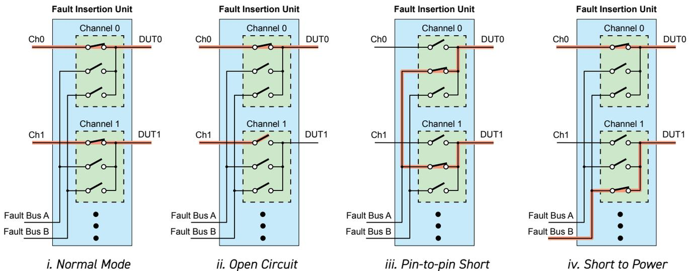
Figure 3. Open & Short Fault Simulation
