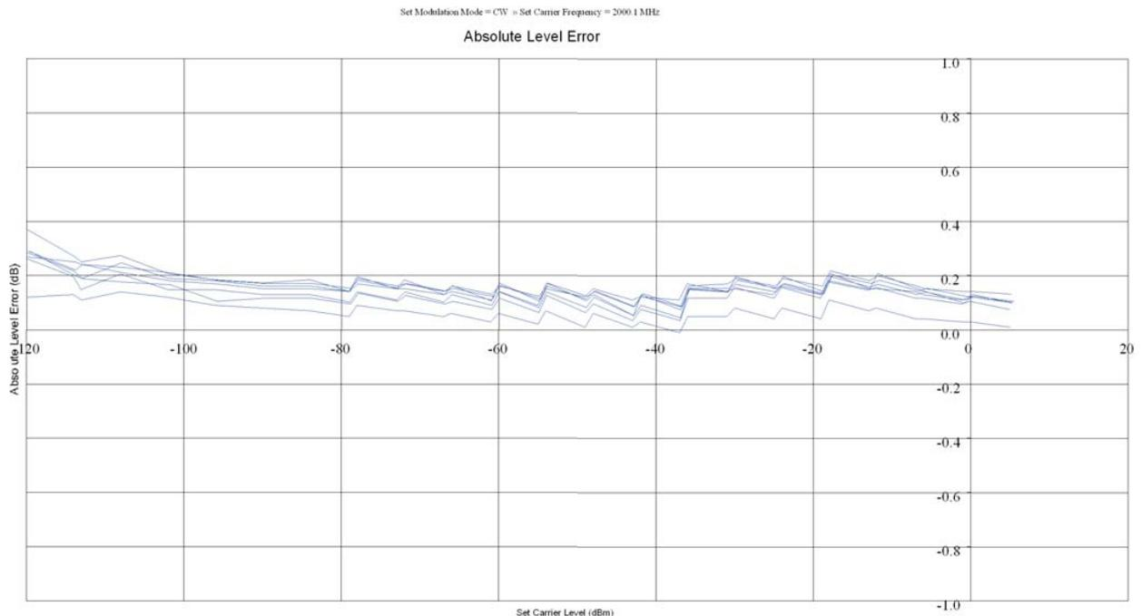
*Figure 5 - Typical Level Repeatability of PXI Signal Generators*
