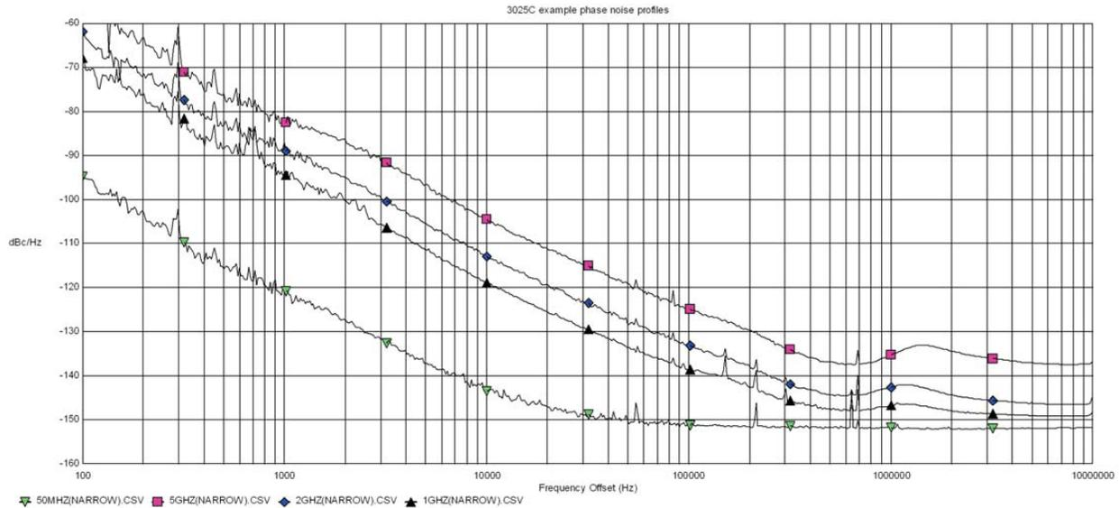
Figure 4 - Typical SSB Phase Noise Performance of PXI Signal Generators
