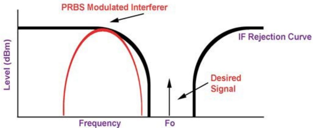
Figure 3 - Adjacent Channel Test
