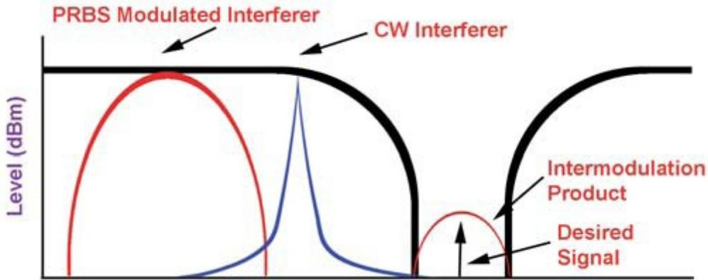
Figure 2 - Intermodulation Blocking Test
