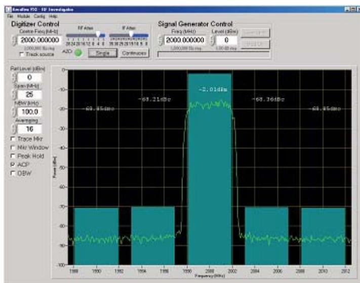
*Figure 6 - Typical ACP Response of PXI Digitizers (3gpp, TM1, 64ch)*
