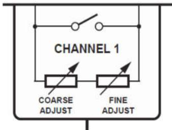
A precision resistor costs more than a standard resistor chain and may have fewer channels because of the added circuitry. But if the application demands this kind of accuracy, there are choices in the market.
