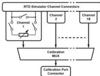
If high-accuracy settings are required, look for resistor modules with a calibration port. In the schematic seen in figure 7, the calibration port is a multiplexer that switches the port to each channel, one at a time. Connecting a precision DMM to the port allows the user to verify the value of every setting required for their test program.
