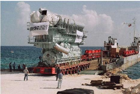
Here is a photo of a very large diesel engine (55,000 horsepower) designed for oceangoing ships. The German manufacturer was planning to test the Engine Management Unit. This module controls the fuel injection based on throttle position and other factors. Of particular interest was the monitoring of the engine block temperature. As this is a very large engine -- as you can tell by the people standing at the base -- they had to monitor 144 temperature probes.
