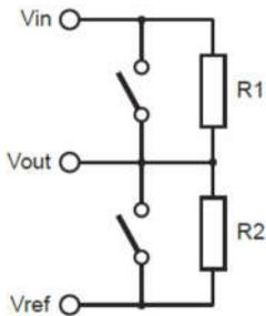
Some versions of programmable resistors include two relays per resistor to inject faults into the test program. These relays can simulate a sensor short or an open. Remember that a fixed-value resistor module may be dedicated to one application only. While a resistor module with a broad resistance range may cost more, it can be more easily reused for future applications.
