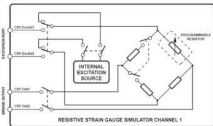
Finally, there are programmable resistor modules configured for a particular sensor type. The two most popular simulate an RTD (Resistive Temperature Detector) or the resistor bridge circuit in a strain gauge. These modules will have software drivers that allow you to set temperatures or program the value required to balance the bridge, and the setting of the simulator can be varied above and below this value to simulate extension and compression of a strain gauge (see figure 6).
