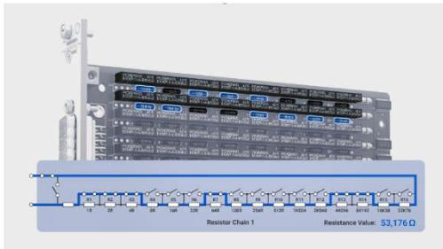
In figure 2, you see a PXI-based programmable resistor module (Pickering Interfaces' model 40-295, similar models are available from several vendors) based on relay chains. If we take a single channel, we see that it is composed of multiple resistors with individual relays connected across them. When all the relays are closed, the series resistance is effectively zero ohms. In actuality, it can be a few hundred milliohms, as each relay and the PCB itself will exhibit a very low resistance.
