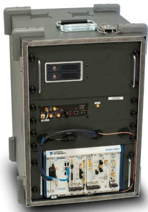
Figure 3 – RF Shielded Box Protects against Interference
