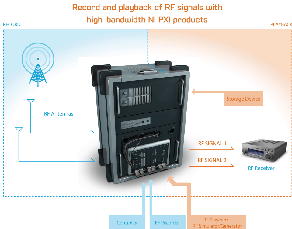
Figure 1 – Record and Playback of RF Signals with High-Bandwidth NI PXI Products
